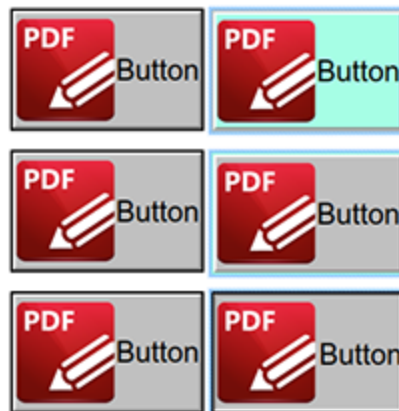
Figure 6. Default to Invert (Top), Default to Outline (Centre) and Default to Push (Bottom)
