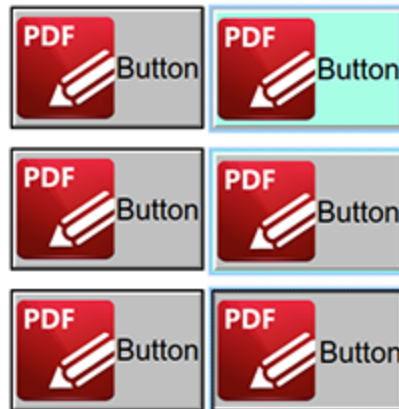
Figure 6. Default to Invert (Top), Default to Outline (Centre) and Default to Push (Bottom)
